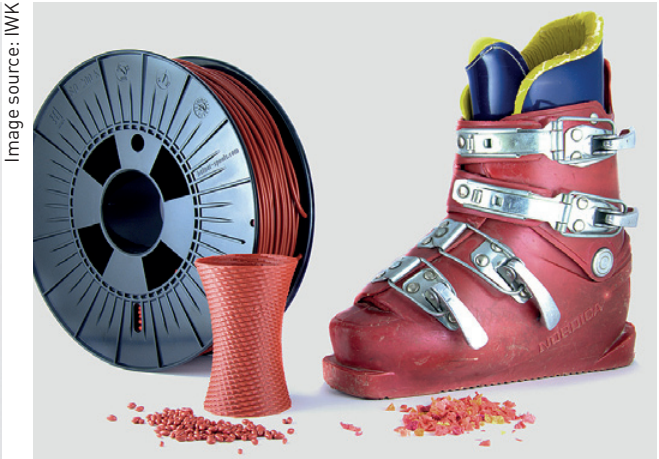
3 Recycled TPU filament made from old ski boots
