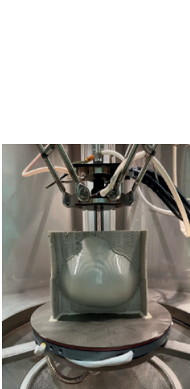
1 Material extrusion 3D printed PEEK cranial implant with support structures (in situ)
