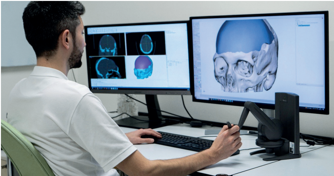
2 In-house 3D designing process for customized cranial implants
